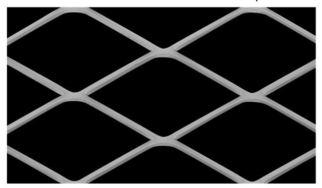
LW Pitch:101.60mmStrand Width:5.03mmSW Pitch:50.80mmThickness:3.00mmWeight:4.66 kg / m2 (Black Weight)Open Area:80%
